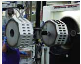
5 Vacuum Metallizing Reflector Machines
