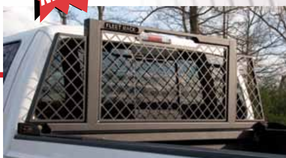
Base model with center window and wing screen guards
